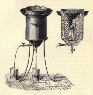
forces. In the improved form, as designed by Bunsen and others, the middle vessel is *filled* with solid ice to begin with, and the amount melted is calculated from the *diminution of the volume* (§ 145) *of the contents*, as shown by an external gauge containing mercury in contact with the ice.
